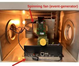
Edge device: Brainchip Akida RaspberryPi board and event-based neuromorphic camera
