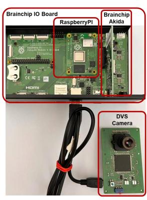
End-to-end pipeline – System hardware
