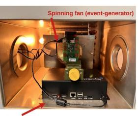
Edge device: Brainchip Akida RaspberryPi board and event-based neuromorphic camera
